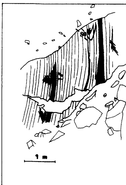
Fig 13 Field observation in the Rosebery open pit traced from photograph (co-ordinates 5,374,675 mN, 378,640 mE, AMG grid). Ore lenses (black) parallel the S_2F_3 -cleavage (thin lines) and cross-cut folded bedding ( S_0 ; heavy lines)
